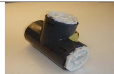
Figure 3. Failure crack in a 2-in. Schedule 80 tee
