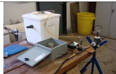
Figure 2. 2-in. Surge Guard PVC tee installed in the test jig with related components
